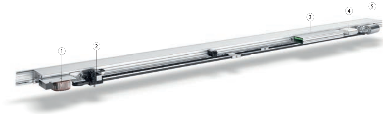
1 = Transformateur | 2 = Verrouillage | 3 = Commande | 4 = Accumulateur | 5 = Moteur
